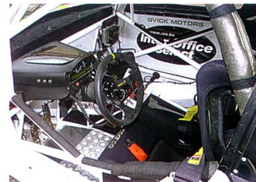
● The driver sits a long way back in Belcar MINI behind three-litre 365bhp M3 straight-six. Scoops, louvres, ducts and huge rear wing are all crafted by Qvick from composites
