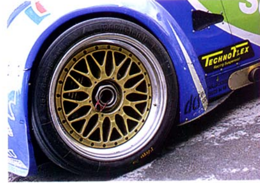
● ATL racing fuel filler, Techno Flex racing suspension with in-board dampers and 10x18-inch slick-shod wheels show the team's serious intent. Chassis still needs work though
