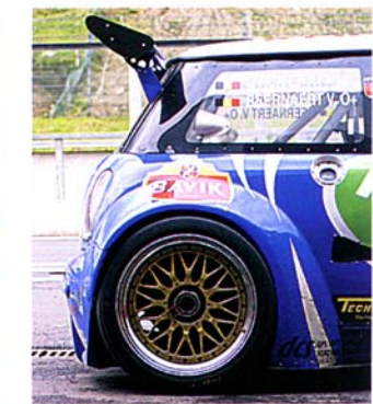
● The driver sits a long way back in Belcar MINI behind three-litre 365bhp M3 straight-six. Scoops, louvres, ducts and huge rear wing are all crafted by Qvick from composites
