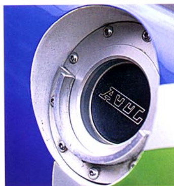
● ATL racing fuel filler, Techno Flex racing suspension with in-board dampers and 10x18-inch slick-shod wheels show the team's serious intent. Chassis still needs work though
