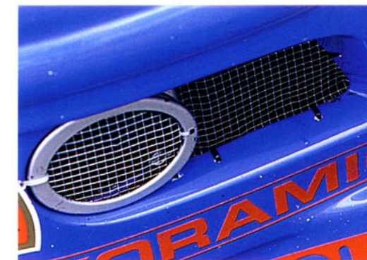
● The driver sits a long way back in Belcar MINI behind three-litre 365bhp M3 straight-six. Scoops, louvres, ducts and huge rear wing are all crafted by Qvick from composites
